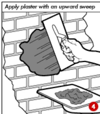
Carry the hawk to the wall and hold it in front of the area you want to plaster. In one movement, tip the hawk towards you, lift off an amount of plaster with the edge of a steel plasterer's trowel and press the plaster against the wall with an upwards sweep of the trowel (4).
