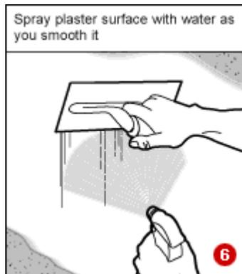
Allow the plaster surface to harden (but not completely dry) before dampening it and smoothing it flat with the trowel (still held at a slight angle) (6). If you are applying a finishing coat, scratch the surface of the undercoat with the edge of the trowel to provide a 'key'.
